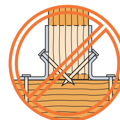
Shorter nails may not be used as double shear nails
